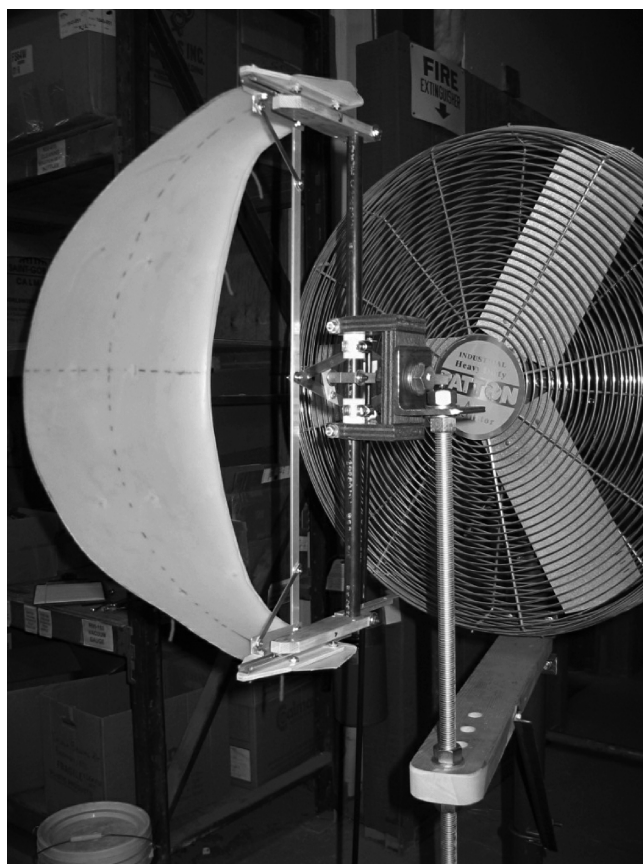
Fig. 9 Setup for arc wing incidence control tests.
