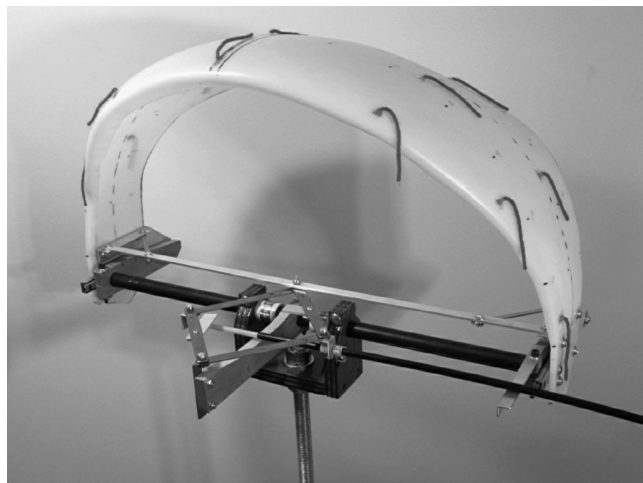
Fig. 8 Arc wing fitted with remote shift mechanism.
