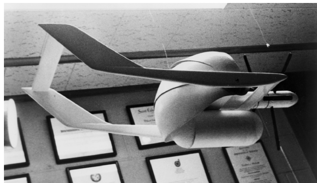
Fig. 1 Arcoputer VTOL static model, flaps extended.
