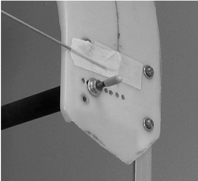
Fig. 3 Wing tip detail with holes for incremental shifts.
