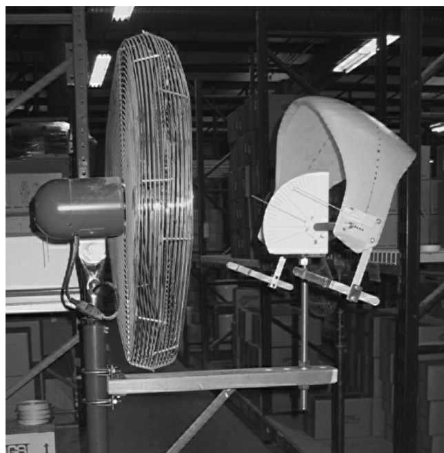
Fig. 2 Pedestal fan and arc wing support structure with angle-of-attack meter.
